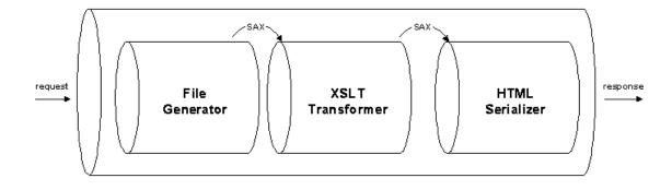
Figure 5: Cocoon Pipeline (Source - http://cocoon.apache.org/2.1/userdocs/concepts/367.daisy.img)
